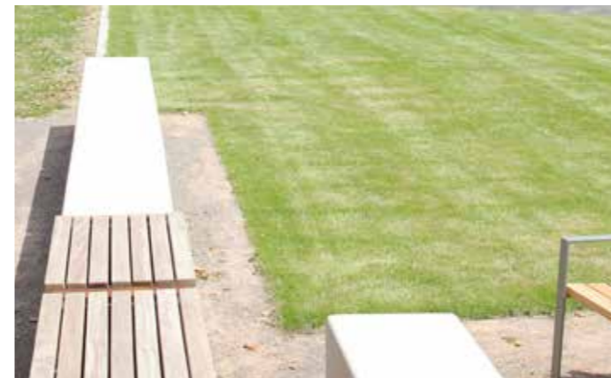
Low walls and incidental seating will reduce the need for bollards and / or traveller defence bunds.
